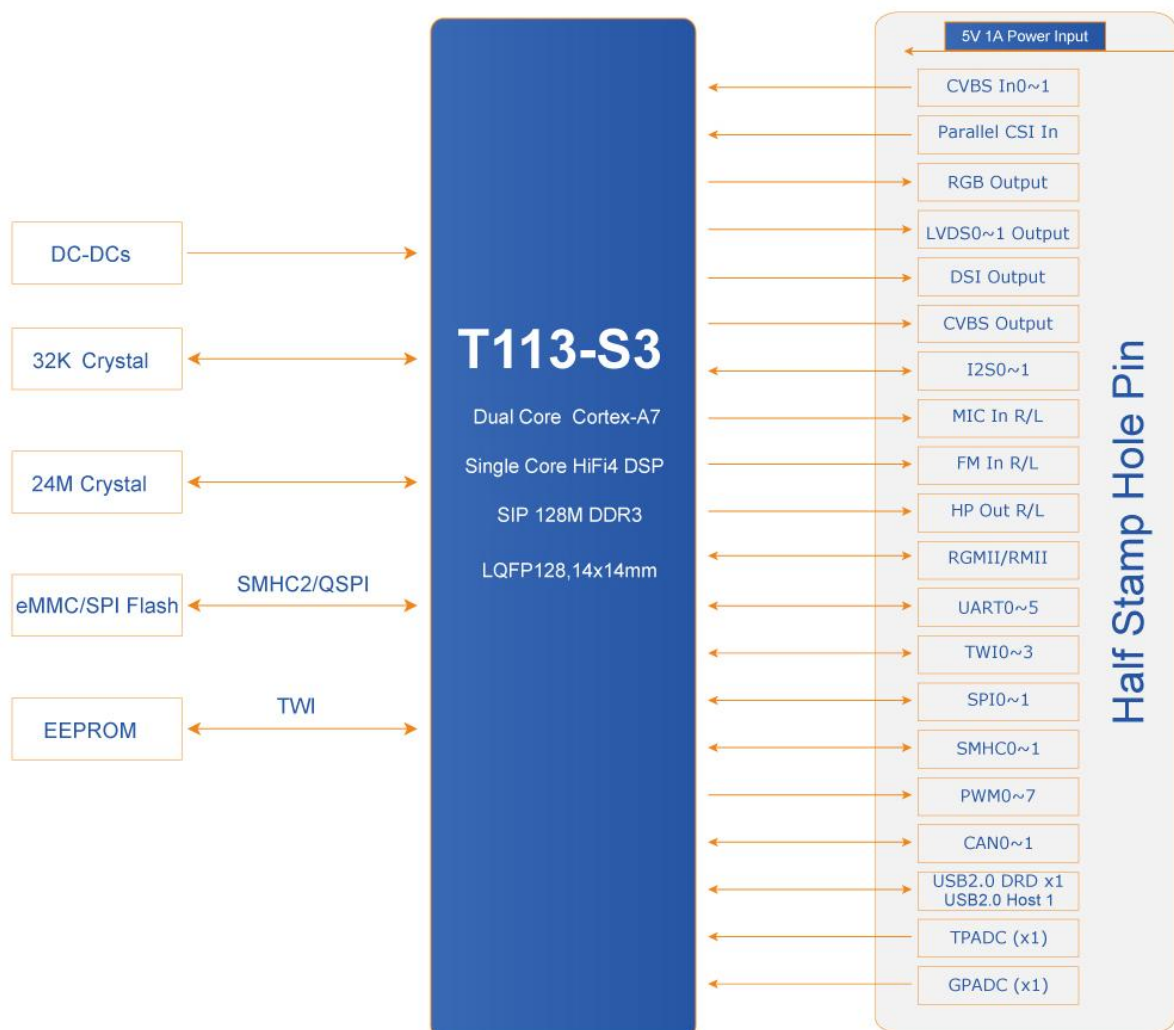
MYC-YT113X Function Block Diagram
