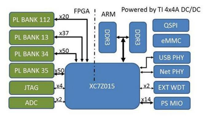
MYC-C7Z015 CPU Module Function Block Diagram
