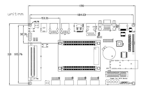
Figure 1-10 Dimensions of MYD-C7Z010/20 Development Board
