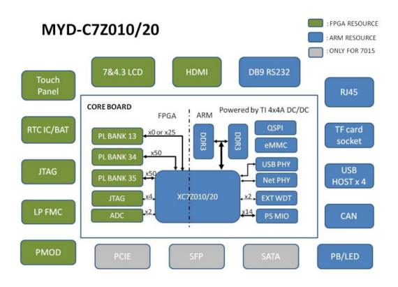
Figure 1-8 MYD-C7Z010/20 Development Board Function Block Diagram
