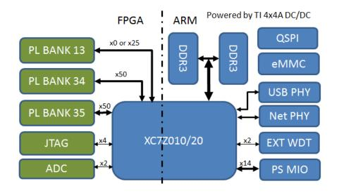
Figure 1-7 MYC-C7Z010/20 CPU Module Function Block Diagram
