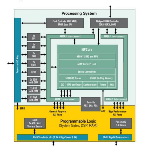
Zyng Z-7000S SoC Device Block Diagram
