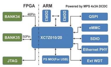
MYC-Y7Z010/20-V2 Function Block Diagram
