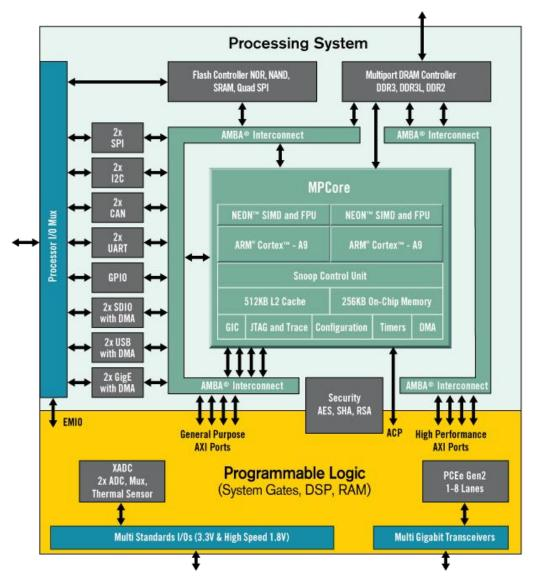
Zyng Z-7000 SoC Device Block Diagram
