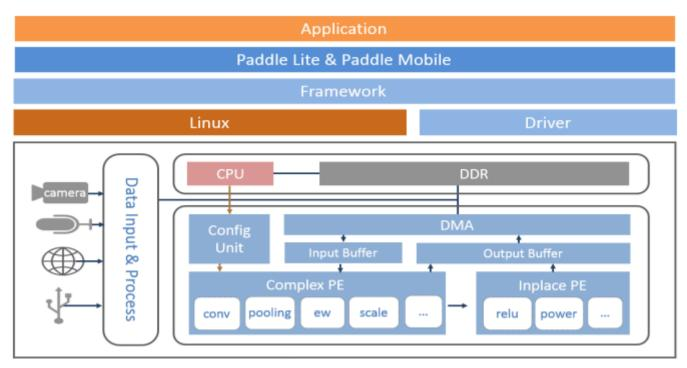
Figure 1-10 Software Architecture of FZ5 EdgeBoard AI Box
