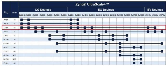
Figure 1-12 Zynq® UltraScale+™ MPSoC Device Migration Table
