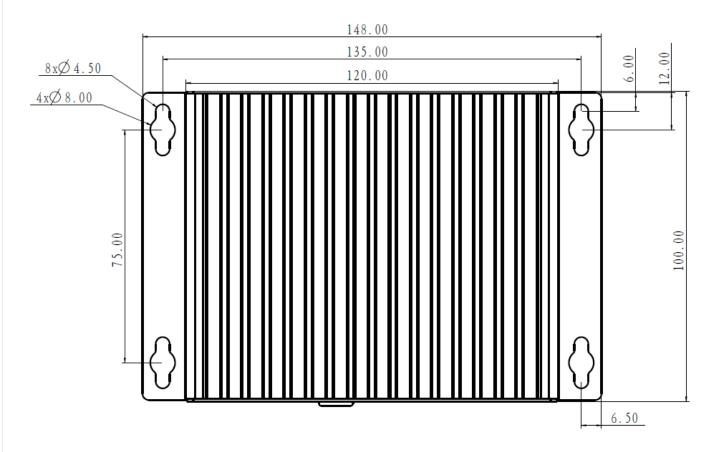
Figure 1-13 Dimension Chart of FZ5 EDGE AI BOX (Unit: mm)
