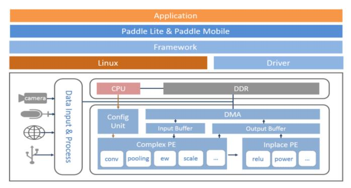
Figure 1-8 Software Architecture of FZ5 Card
