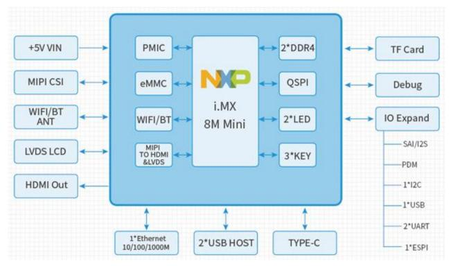
Figure 1-7 MYS-8MMX-V2 Function Block Diagram
