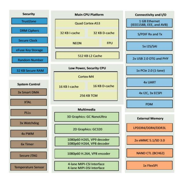
i.MX 8M Mini System Block Diagram
