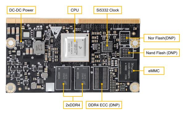
MYC-J1028X CPU Module Top-view (delivered with heatsink by default)
