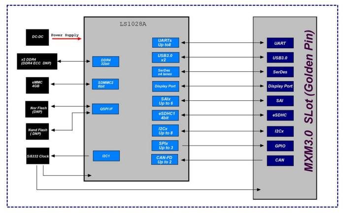
MYC-J1028X CPU Module Function Block Diagram
