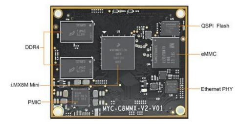
MYC-C8MMX-V2 CPU Module Top-View
