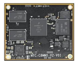
✓ NXP i.MX 8M Mini Quad Application Processor based on 1.8 GHz Arm Cortex-A53 and 400MHz Cortex-M4 Cores
