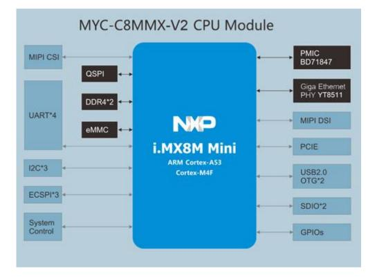
MYC-C8MMX-V2 CPU Module Function Block Diagram
