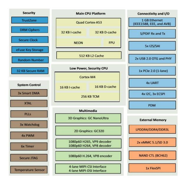
i.MX 8M Mini System Block Diagram
