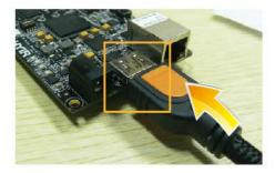
Connect the Z-turn Board J4 to a monitor through an HDMI cable.
