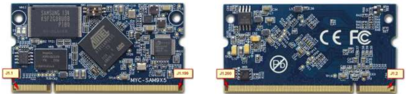
MYD-SAM9X5 Development Board (using MYC-SAM9X5 as controller board)
