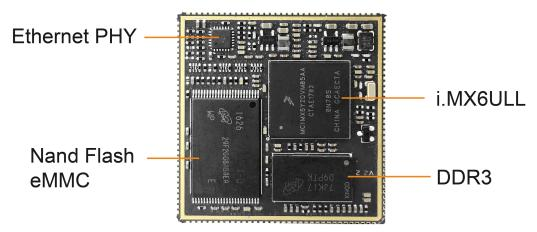
MYC-Y6ULX-V2 CPU Module Top-view (delivered with shielding cover by default)
