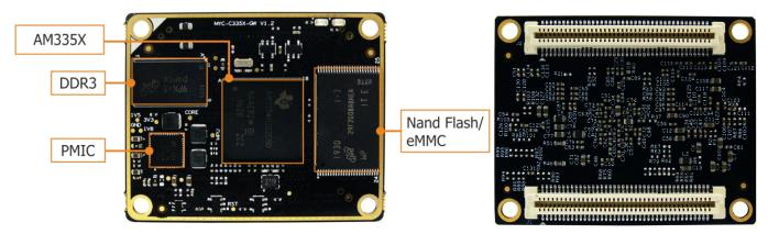
MYC-C335X-GW CPU Module (Top-view and Bottom-view)
